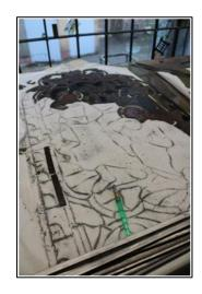
When the window arrives in the workshop, the lead is marked with 'heelball' wax. The outline image of the window can then be transferred to sheets of paper. The
