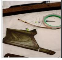
copper tape which is then soldered into place. The resulting join will only look like a line on the finished window. Where the glass is in a very bad state, a new piece will be selected. The range of glass held in the workshop was very comprehensive both in style, colour
