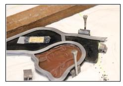
When the window is complete, the lead is soldered together, and special filler inserted carefully around each piece so that it fits tightly together. This also makes the windows watertight.
